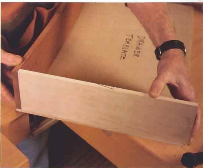
Check the angle. Use the template to see if the drawer front and side meet at the correct angle.
