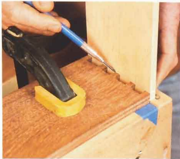
Marking the tails. With a drawer side resting on the paring platform and pressed against the drawer front, use a sharp pencil or a knife to mark the location of the tails.
