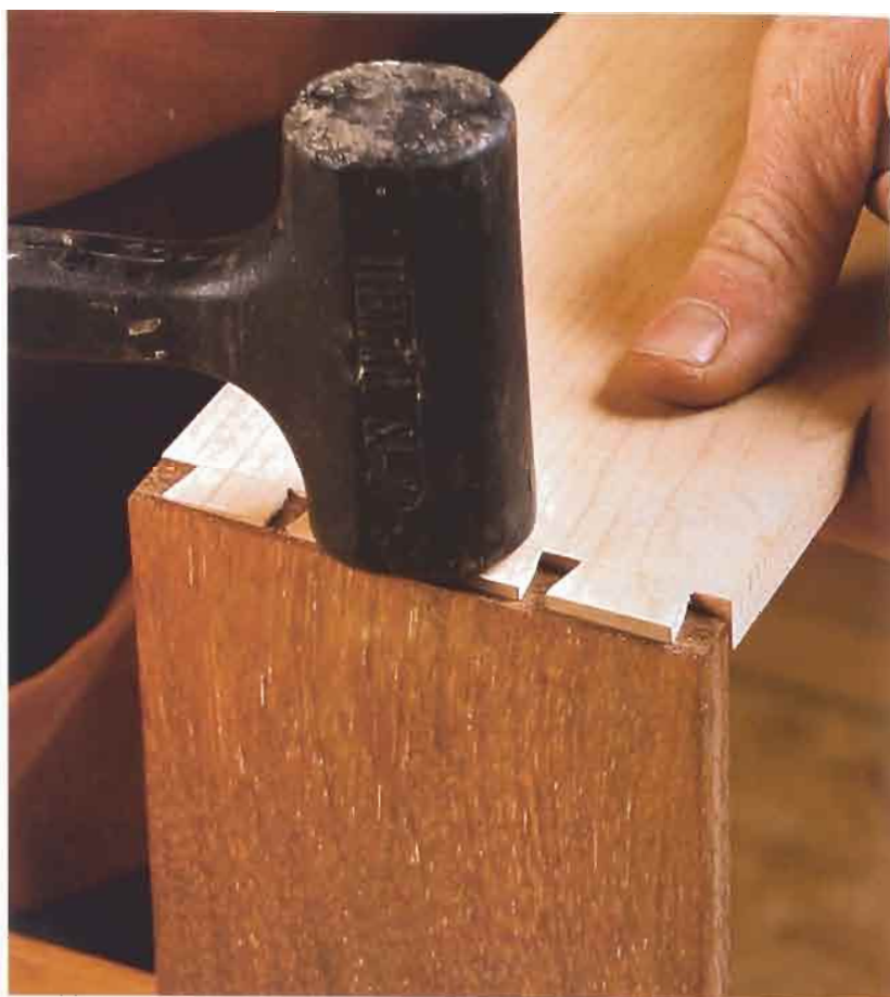
A perfect fit. The secret to well-fitting dovetails is to gradually pare away small amounts of wood, checking the fit regularly.
