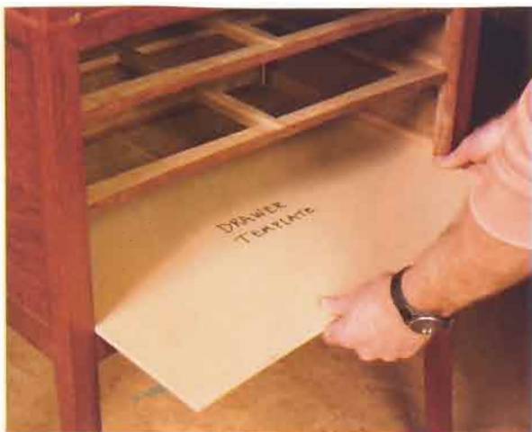
A working template. Create a template from 1/4-in. MDF that exactly fits the drawer opening and the profile of the drawer front. This will reveal the angle at which the drawer sides enter the drawer front.
